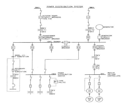
Figure 1: Typical One-Line Diagram
